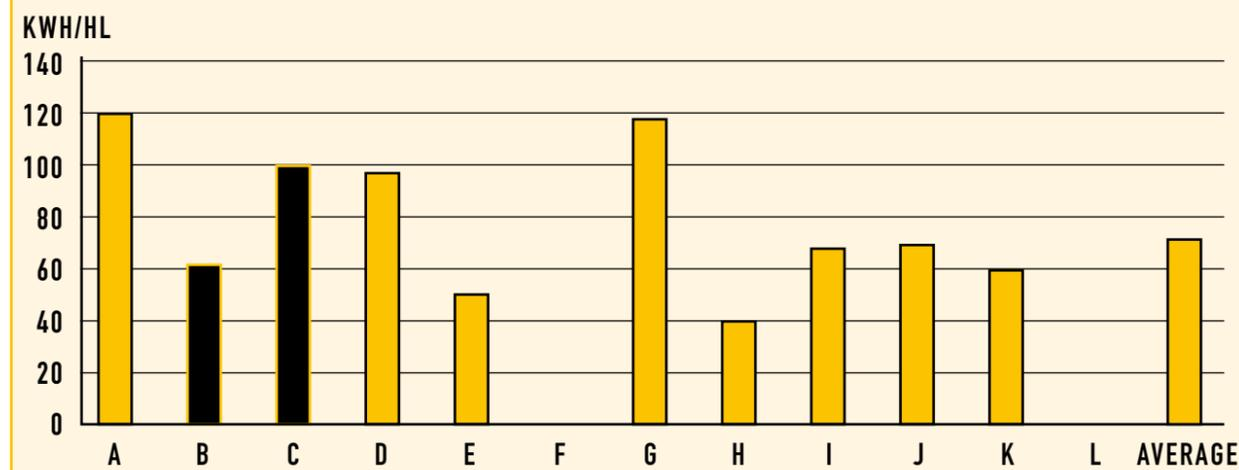
Total energy consumption for heat and electricity in kWh/hl from 10 of the 12 microbreweries in the survey for 2011. Black columns represent breweries without small pack filling lines.
